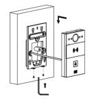
Insert the four wall-mounting screws on the device into the corresponding holes on the wall-mounting bracket, and then press down to slide the wall-mounting screws into the groove. Then use the Allen Wrench to tighten the device with two M3x6 screws.
