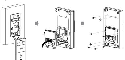
For convenient wiring, hang R20A on the wall-mounting bracket with rope.
