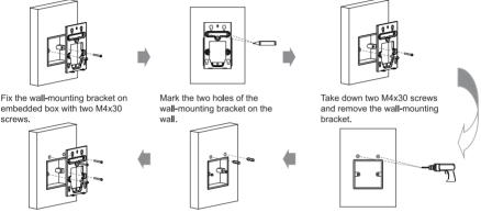
Fix the wall-mounting bracket with two ST4x20 screws and two M4x30 screws.
